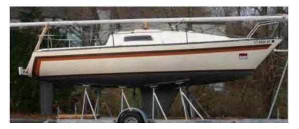
The Sj 7.7 is 'trailerable', but as with any boat with a 4 ft draft and over 9 ft beam, prudence and the proper permits are required. Around 210 San Juan 7.7's were made over is production run, many with the inboard OMC saildrive propulsion. A few were outfitted with single cylinder 7 hp diesel inboards.
