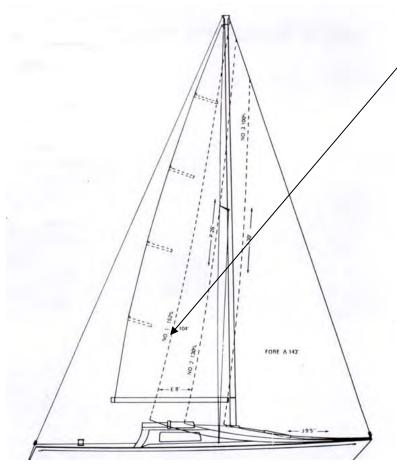
The rig was typical of IOR masthead rigs of the time – short Boom, and big fore triangle. The San Juan 24 was one of the first to use the swept-back spreaders to help lock the mast in and help the backstay provide really good tension on the forestay.
